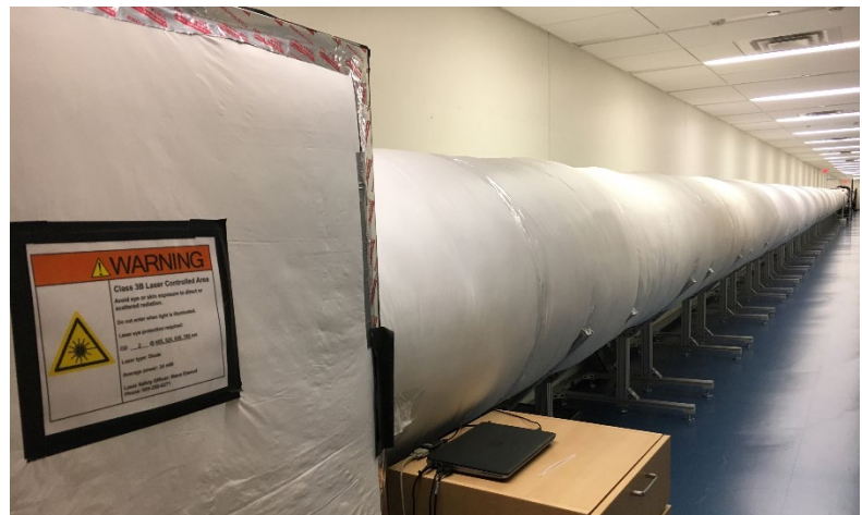
Figure 2: Princeton Starshade Testbed located on campus. This 80 meter long, 1 meter diameter tube provides a clean and dark environment for conducting optical tests on the starshade masks. Data from this experiment are used to validate optical models predicting the starshade's starlight suppression capabilities.
