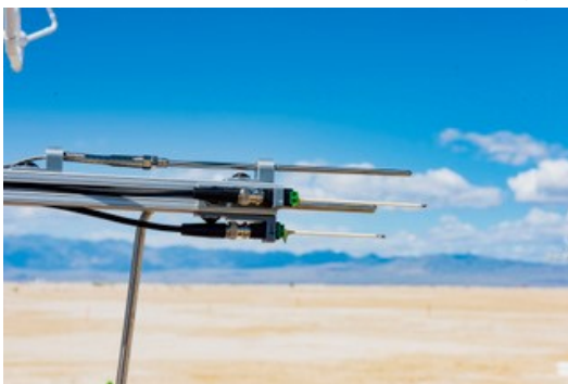
Figure 1: One station of the set-up deployed at Utah's SLTEST facility. An NSTAP, a TNSTAP, a pitot tube, and a thermocouple are mounted.
