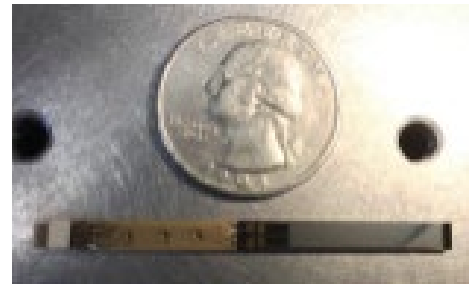
Figure 2: Large-area MOSFET for electron spin resonance measurements, fabricated in the PRISM cleanroom.
